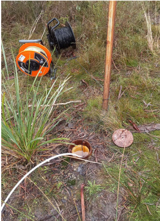
North-western downgradient bore showing water level at ground level (BH2)
